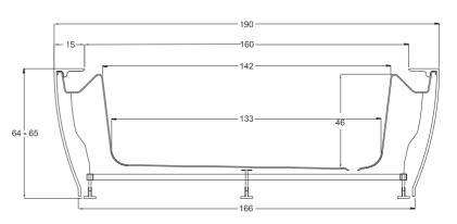
If the bath is recessed the masonry cannot reenter more than 1 cm with respect to the external edge of the bath. An inspection panel and air intake must be installed.
